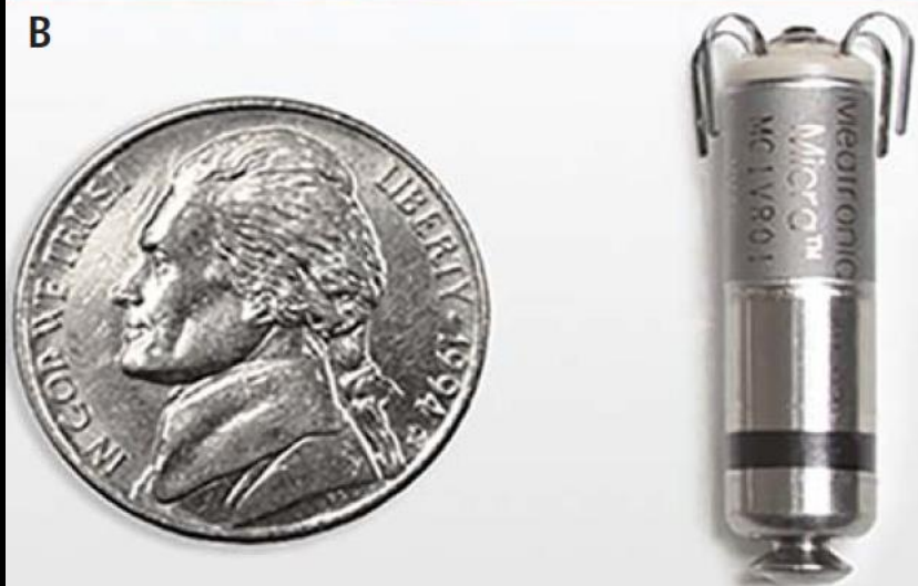
FIGURE 2. Leadless pacemakers (A) Nanostim and (B) Micra.
